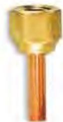
PART # CD2594 PKG QTY: 2 A 1-1/4" piece of 1/4" copper tubing, double flared on one end with a 1/4" female flare nut and a depressor tip.
