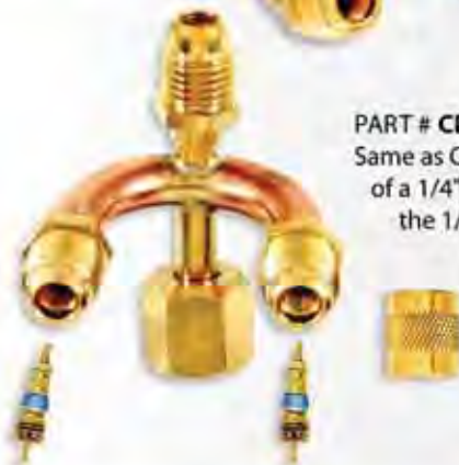
PART # CD2595 PKG QTY: 2 The same as CD2594, only the end of the copper tube opposite the female flare has been swaged to allow 1/4" copper tube inserted for brazing.
