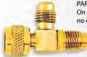
PART # CD8725 PKG QTY: 2 The CD8725 has a gasket in the 1/4" hex nut. The valve body is stationary. When threads of existing system fittings are stripped and a new core won't go in, use this. It has a core and no depressor tip.
