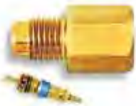
PART # CD1450 PKG QTY : 2 1/4" flare access x 1/4" f. flare adapter, with one valve core and copper gasket.
