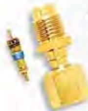
PART # CD8725 PKG QTY: 2 The CD8725 has a gasket in the 1/4" hex nut. The valve body is stationary. When threads of existing system fittings are stripped and a new core won't go in, use this. It has a core and no depressor tip.
